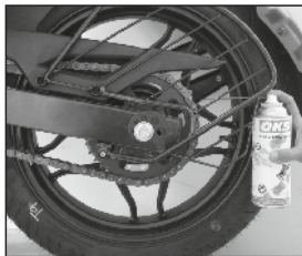
Drive Chain Lubrication
